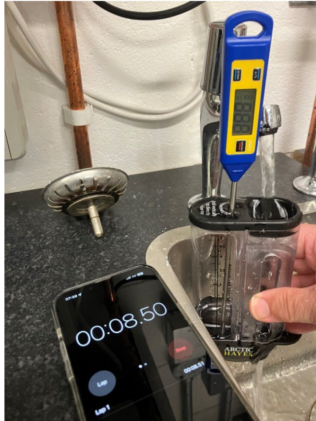
Fig 14 – measuring DHW flow rates, temperature and time to reach outlets (image Bosch).
